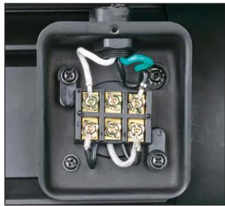
Figure 66. Bandsaw motor wiring.
